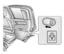
The vehicle has rear door safety locks on each rear door that prevent passengers from opening the rear doors from the inside.
