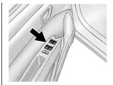
The switches on the driver door control all windows. In addition, each passenger door has a switch for its own window.
