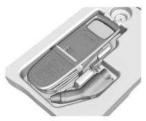
Open the rear hatch, lift the load support floor covering, and remove the charge cord. It is located near the tire sealant and compressor kit. Pull up on the charge cord
