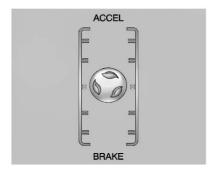
This gauge is a guide to driving in an efficient manner by keeping the ball green and in the center of the gauge. The leaves stop spinning when the vehicle stops or when the ball travels away from the center of the gauge.
