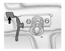
Go to the front of the vehicle and push the secondary hood release lever up.
