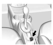
Sport Mode provides more responsive acceleration than Normal Mode, but can reduce efficiency. Use Normal Mode whenever possible. When the SPORT light is not on, the vehicle is in Normal Mode.
