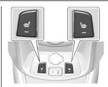
The buttons are below the climate control system. To operate, the vehicle must be on.
