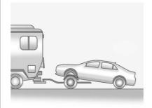
Tow the vehicle with the two rear wheels on the ground and the front wheels on a dolly.
