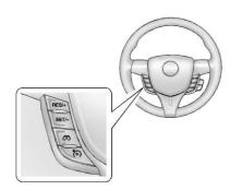
(On/Off): Press to turn the cruise control system on and off.
