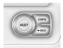
**CONFIG**: Press to change the instrument cluster display configuration. See *Instrument Cluster* ⇒ 94.
