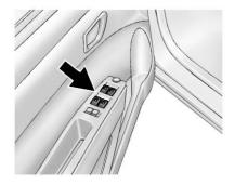
Press the switch down to open the window. Pull the front of the switch up to close it.
