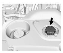
Check to see if coolant is visible in the high voltage battery coolant reservoir. If coolant is visible but the coolant level is below the cold fill line, there could be a leak in the cooling system.
