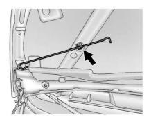
Lift the hood and release the hood prop from the prop retainer, which is under the hood.
