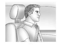
Adjust the head restraint so that the top of the restraint is at the same height as the top of the occupant's head. This position reduces the chances of a neck injury in a crash.
