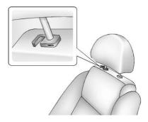
The vehicle has a shopping bag hook under the front seat head restraints. Lift the head restraints to access the hook.
