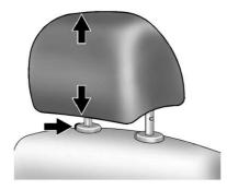
The height of the head restraint can be adjusted. Pull the head restraint up to raise it. Try to move the head restraint to make sure that it is locked in place. To lower the head restraint, press the button, located on the top of the seatback, and push the head restraint down. Try to move the head restraint after the button is released to make sure that it is locked in place.
