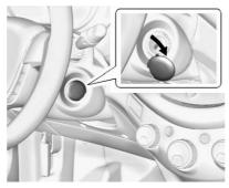
Remove the rubber cap on the steering column. Press the button on the new transmitter to extend the key blade. Insert the key blade into the transmitter slot.
