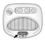
The dome lamp controls are in the overhead console.
