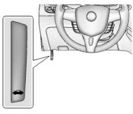
Pull the hood release handle inside the vehicle. It is on the lower left side of the instrument panel.
