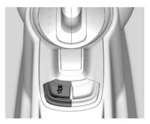
The button for TCS and StabiliTrak is on the center console behind the shift lever.
