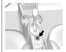
The vehicle has an Electric Parking Brake (EPB). The (P) switch is on the center console. The EPB can always be activated, even if the vehicle is off. To prevent draining the 12-volt battery, avoid repeated cycles of the EPB system when the vehicle is off.
