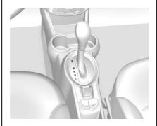
**P**: This position locks the front wheels. It is the best position to use when starting the propulsion system because the vehicle cannot move easily.
