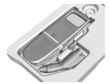
Open the rear hatch, lift the load support floor covering, and remove the charge cord. It is located near the tire sealant and compressor kit. Pull up on the charge cord
