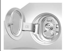
Plug in the AC vehicle plug of the charge cord into the charge port on the vehicle. Make sure
