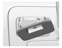
Remove the fuse panel door diagonally.
