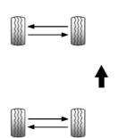
Use this rotation pattern if the vehicle has different size tires on the front and rear.
