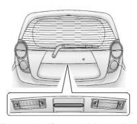
To open the liftgate, pull the handle and lift up.
