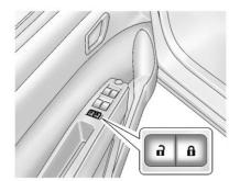
To lock or unlock the liftgate from the inside, press  $\widehat{\ }$  or  $\widehat{\ }$ .
