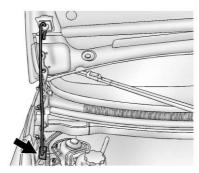
Securely place the hood prop into the hood prop holder, at the rear passenger side of the underhood compartment.
