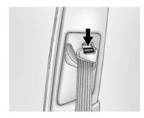
Press the release button and move the height adjuster down to the desired position. The adjuster can be moved up by pushing up on the adjuster.
