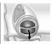
Press the cover of the side air vents to open. Turn open slats clockwise or counterclockwise to direct airflow as needed. Close the cover to stop the airflow.
