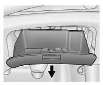
Open the glove box completely and pull it up by each side to remove.
