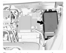
The underhood compartment fuse block is on the driver side of the vehicle, near the battery.
