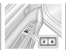
To lock or unlock the doors from inside the vehicle:
