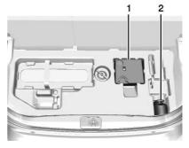
2. Remove the compressor (1) and the tire sealant canister (2).
