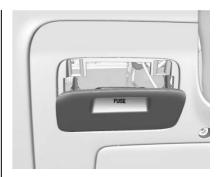
Open the fuse panel door by pulling out at the top.
