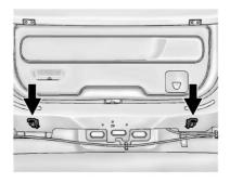
The top tether anchors are on the rear wall of the cargo area. Be sure to use an anchor on the same side of the vehicle as the seating position where the child restraint will be placed.
