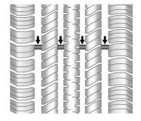
Treadwear indicators are one way to tell when it is time for new tires. Treadwear indicators appear when the tires have only 1.6 mm (1/16 in) or less of tread remaining. See *Tire Inspection* ⇒ 248 and *Tire Rotation* ⇒ 249.
