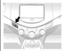
The vehicle has an electronic pushbutton start.
